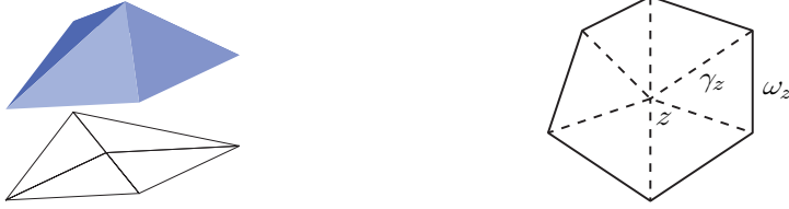
FIG. 1. Example of a test function \varphi_S associated with an interior side S (left) and finite element star \omega_z with skeleton \gamma_z (indicated by dashed lines) for d = 2 (right).
